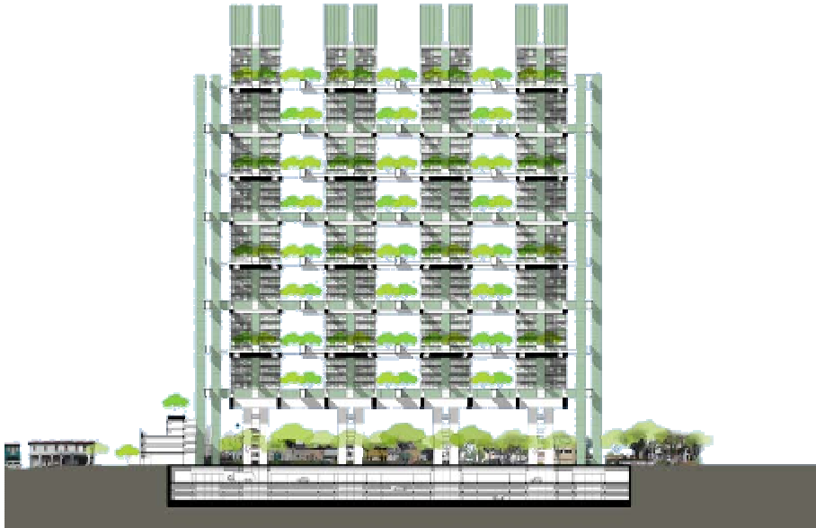
Figure 5 – Section showing the vertical stacking of Shophouse scale Streetscapes
