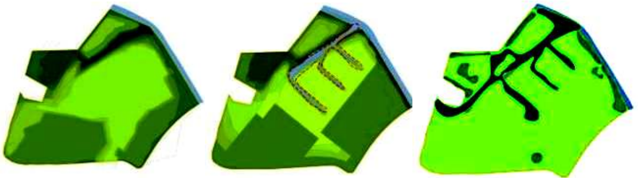
Figure 18 – Diagrams showing the manipulation of site topography which creates the stream gullies that structure the entire masterplan and provide grey water treatment
